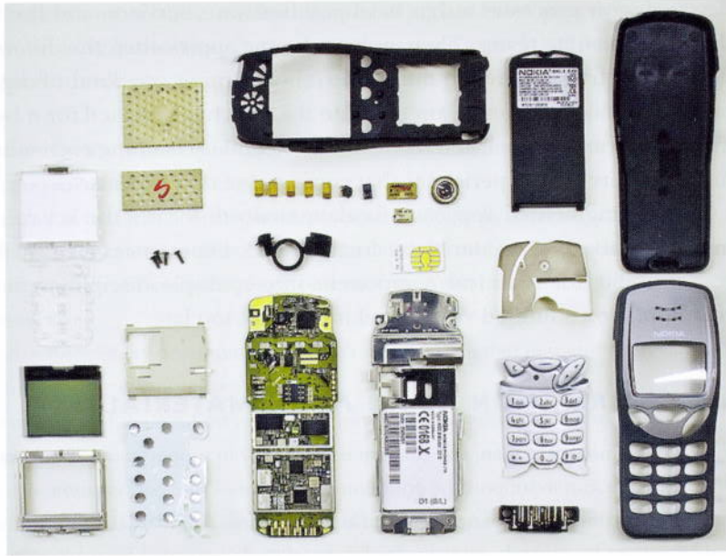
Figure 4-1 A disassembled phone. (Photo © Johannes Henseler, licensed under Creative Commons Attribution 2.0, found on Flickr)
