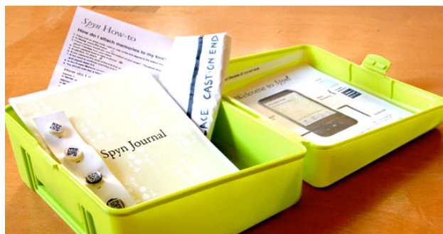
Figure 5. The Spyn "Kit". The kit contained support materials for the Spyn software and a journal for documenting daily activity with Spyn. Support materials included barcode "buttons" (for switching projects), a scanning guide (for gauging the viewfinder's distance from the garment), and instructions for using Spyn.
