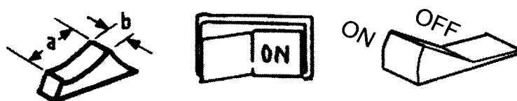
Figure 7.8 Bistable toggle switches (left part from Burandt 1986, middle part from Woodson 1986 and right part from Baumann and Lang 1998).
