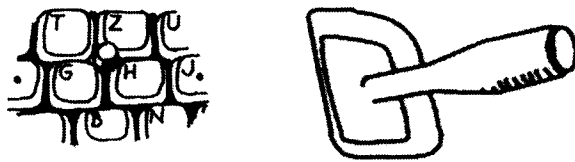
Figure 7.24 (Left) Two-dimensional isometric joystick or trackpoint built into a keyboard; (right) two-dimensional isotonic joystick in a model aeroplane remote control.
