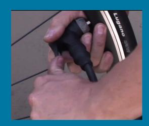
The pump valve head must be applied to the tire valve with both hands, and then fits loosely with no visible confirmation of an airtight seal.
