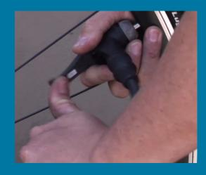
One hand holds the valve head in place while the other hand applies force sideways and away from tire valve, possibly ruining seal between valves and reducing pump efficiency, or even breaking the tire valve.
