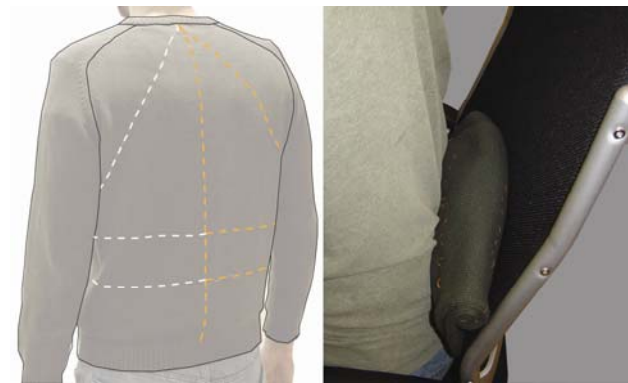
Figure 4. One student with a chronic sports injury created a garment for body awareness - a sweater, stitched with a pattern offering directions for folding into a back support device. Embedded vibrating motors occasionally remind the user to move and reorient his posture.
