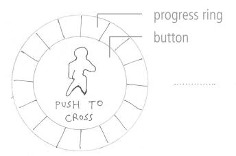
The pedestrian pushes the button, and the progress ring is filled to give immediate feedback. The symbol and the words on the button provide feedforward knowledge.
