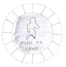
When the ring is gone completely, the pedestrian is able to cross. The system releases the button when the crossing is over.
