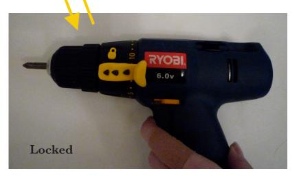
While in use, the thumb trigger is locked down internally and the bit cannot be released. An LED indicator in the shape of a lock shows this.
