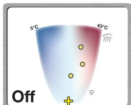
The Digital Shower is a new shower interface based on a touch screen, allowing the user to directly visualize and control the temperature and intensity of the water.
