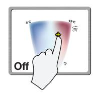
A single finger press on the water space, and the shower will promptly deliver the desired water. Here, the user selected one of the preset points, which are automatically determined by past showering experiences.
