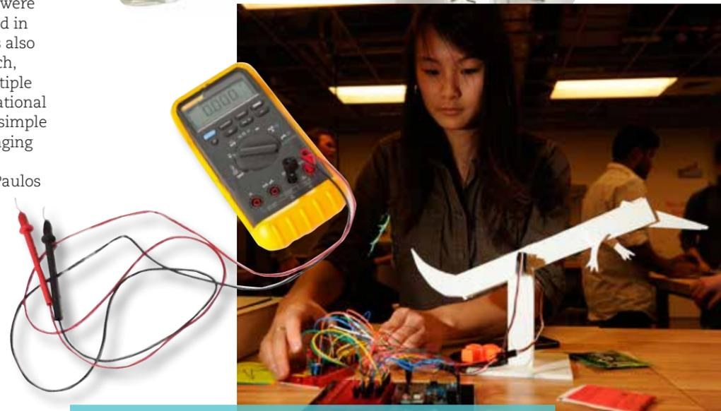
Third-year EECS major, Brittany Cheng, makes some adjustments to Tea-Rex, a device programmed to steep the perfect cup of tea. Motors connected to an Arduino controller raise and lower the neck of the apparatus.
