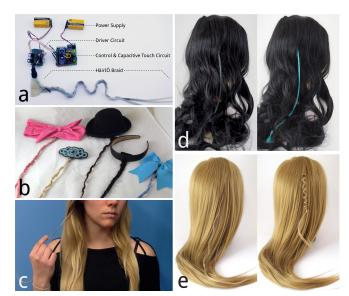
Figure 1. A) HäirlÖ prototype prior to miniaturization, B) exemplar HäirlÖ hair accessory form factors, C) HäirlÖ uses Swept Frequency Capacitive Sensing to detect natural hair interactions, D) HäirlÖ color changing properties using thermochromic pigments, and E) shape changing properties using Nitinol wire.
