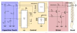
Figure 2. Circuit diagram for our system. The circuit can be extended by connecting additional braids to the available I/O pins of the multiplexer. Note: additional braids require an additional driver circuit. All ground is connected. However, the circuit requires two separate 9V batteries: one connected to the control circuit, the other to the driver circuits.
