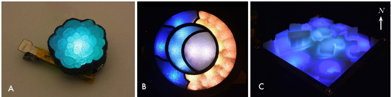
Figure 1. a) an illuminated hairpin (1 led); a tactile flexible diffuser cast with small glass beads creates diffusion and shadow, b) a sun-moon light art piece (25 leds); a computationally generated reflector controls light rays to form soft and hard edges to blend colored lights, c) a dynamic tactile map of an urban center (16 leds); volumetric diffusers indicate building locations; buildings light up in succession to indicate pathways.
