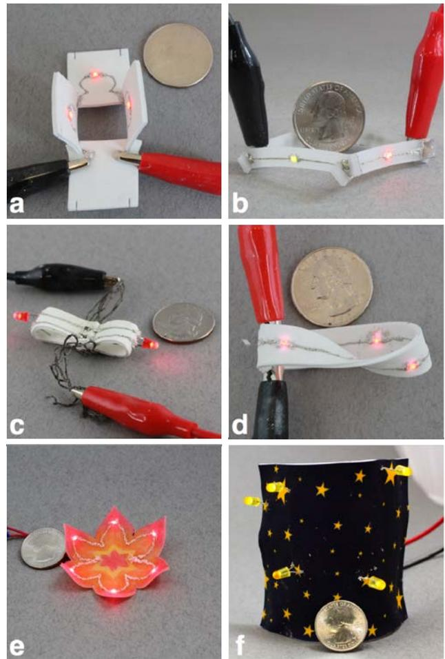
**Figure 8: Non-planar ShrinkyCircuits.** a) A box-like circuit held together by slot cutouts. b) A square frame held together with slot cutouts. c) A bow-tie circuit connected with conductive threads. d) A Möbius strip LED circuit. e) A flower-shaped tealight decorated with color pencils. f) A night light with patterns printed with an inkjet printer.
