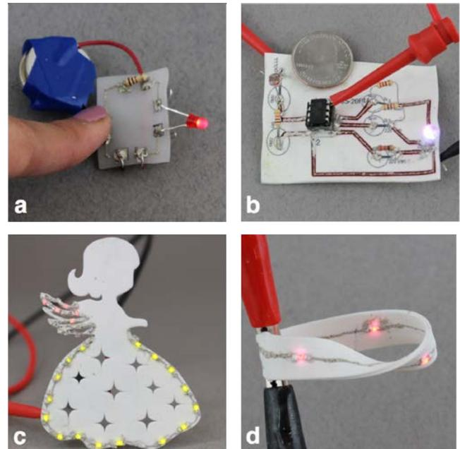
**Figure 1. Different types of ShrinkyCircuits. a) A LED circuit with a physical switch and through-hole electronic components. b) An Eagle generated design with a microcontroller and through-hole components. c) A LED circuit board with fine cutout details made with a low-cost vinyl cutter. d) A Möbius strip LED circuit.**
