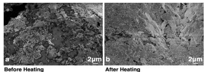
**Figure 2: Scanning electron microscopy (SEM) pictures of the conductive silver ink on a polymer substrate. a) Before the silver ink and the substrate are heated. b) After the silver ink and the substrate are heated.**
