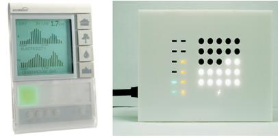
**Figure 4.** The EcoMeter (left) and local energy display (right).
