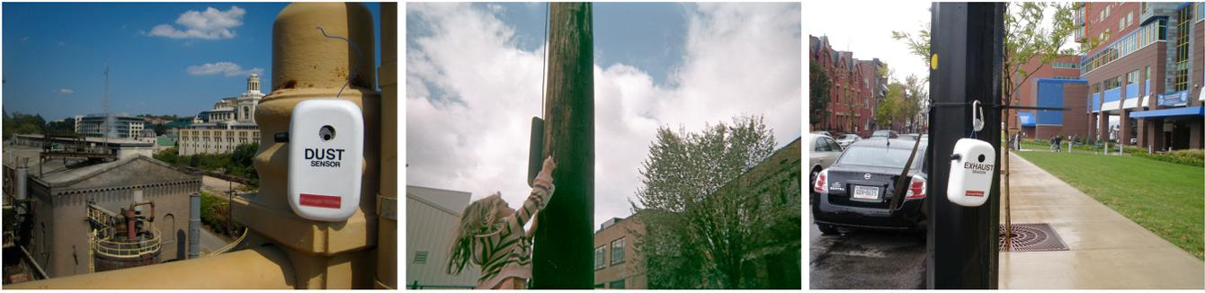
**Figure 4. Photographs of participant sensor placements: dust sensor attached to bridge by bicyclist (left), participant's daughter attaching VOC sensor to street pole (middle), and exhaust sensor outside a children's hospital placed by activist (right).**
