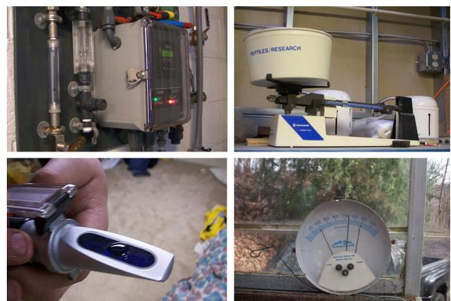
**Figure 2. Technologies used by participants: ORP probe, routinely used to monitor ozone levels in aquariums (top left), scale for weighing reptiles (top right), refractometer, occasionally used to check honey before harvesting (bottom left); thermometer, checked daily (bottom right).**
