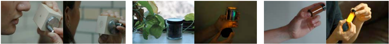
Figure 2. Energy Memento prototypes (left to right). Crank-Sound Box . Turning the crank on one face records sound using energy collected from cranking; turning the crank the opposite direction plays the recorded sounds through the speaker on the opposing face. Light Jar . The jar collects solar or other light energy; opening the jar activates the energy as a glowing light. Shake-Light Bottle . Shaking the bottle collects energy; removing the cap activates the light energy.
