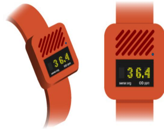
It is not uncommon for people to use Bluetooth headsets (exposed to ambient air) while their mobile phone is in their bag or pocket (not exposed to ambient air). Similarly, we can imagine the use of various Bluetooth based air quality sensors attached to clothing, body, or backpacks for sampling the ambient atmosphere. We are also in the process of developing a wristwatch version of the hardware with a numeric output on a watch face. A sketch of this design concept is shown (Figure 7).
