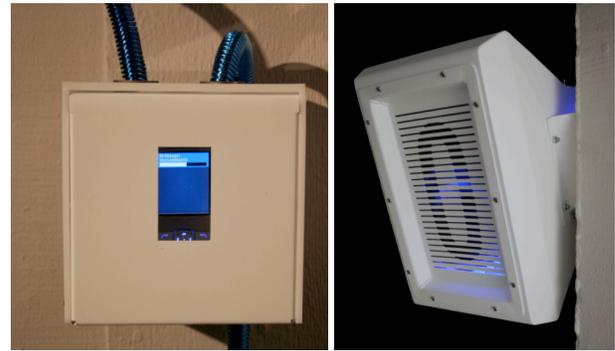
**Figure 3:** Hullabaloo mobile phone enclosure box (left) and speaker box (right)
