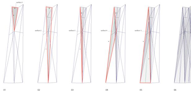
**Figure 4.** The four distinct folded cutouts that form the language for building the overall tessellated surface. Deeper tessellated patches are used in regions of unexpected behavior
