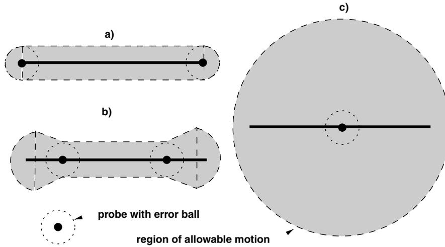
Fig. 4. Relationship of placement of probes (solid points) with error balls (dashed circles) along an edge (solid line) and the resulting displacement region (shaded): (a) probes at endpoints of the edge, (b) probes moved inward from the edge resulting in a larger region of allowable motion, (c) probes coincident at the center of the edge, allowing a maximum displacement region.
