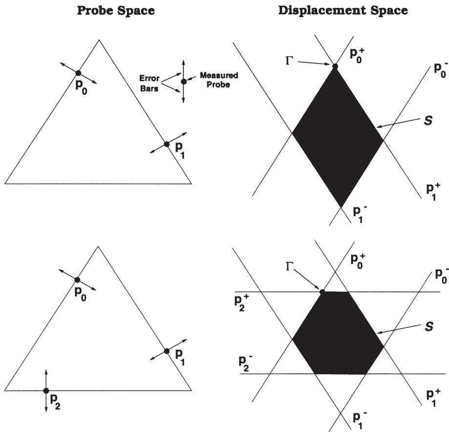
Fig. 6. Simple example of probe space and displacement space without considering rotation. Note the removal of one probe and the resulting change of the polygon  $S$  in the displacement space.
