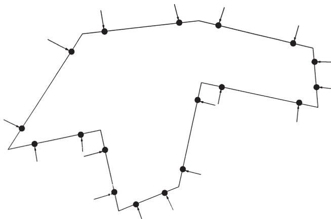
Fig. 2. Typical initial probe placement along the edges of an object.
