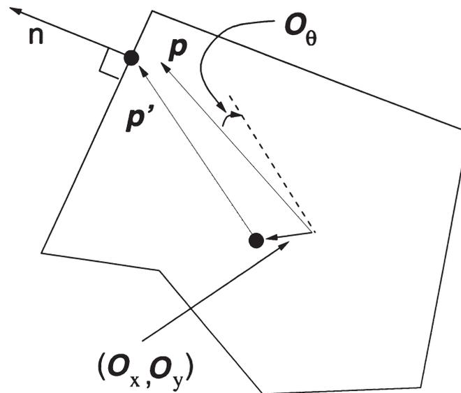
Fig. 5. Original probe  $p$  and resulting probe  $p'$  after an object displacement  $(O_x, O_y, O_\theta)$ .
