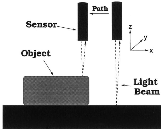
Fig. 1. A typical simple reflective sensor used for probing.
