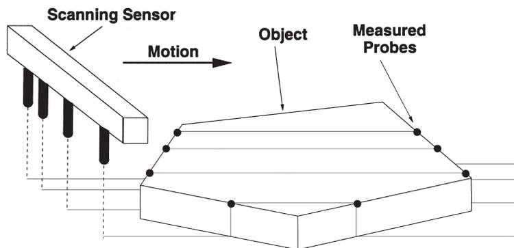
Fig. 3. Example of a fixed-array scanning beam sensor.
