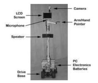
**Figure 4:** A cart **PRoP** with camera head, video LCD screen, controllable "arm/hand" pointer, microphone, speakers, and drive-able base.
