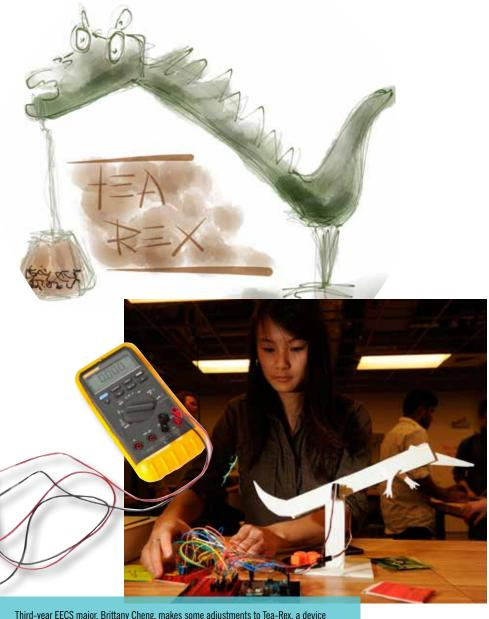
programmed to steep the perfect cup of tea. Motors connected to an Arduino controller raise and lower the neck of the apparatus.
