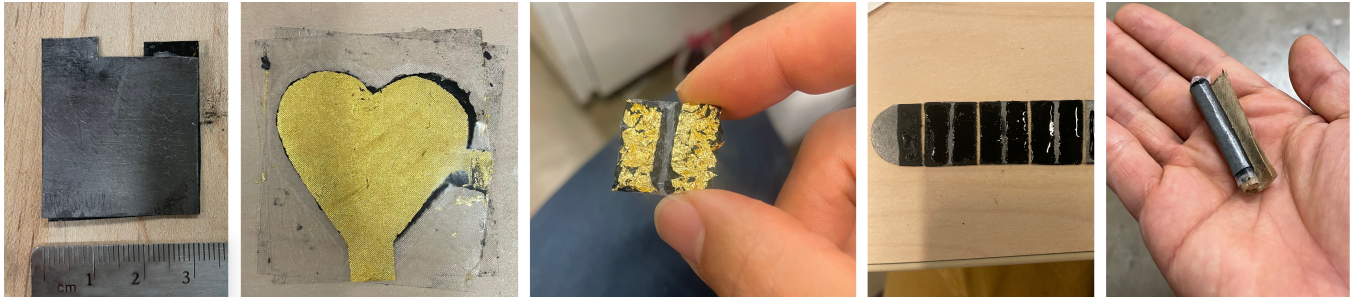
Figure 1: Readily fabricated in a makerspace, VIMs can take a variety of shapes and form factors.
