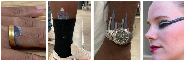
Figure 4: Lotio is a dynamic overlay worn on the skin. When lotion is applied, Lotio functions as a computationally-controllable segmented display, with some portions of the design becoming more saturated and darker in appearance, and other portions of the design becoming less saturated and lighter in appearance. From left to right: “Ocean Waves” prototype on a finger, “Geometric Bear” prototype on a leg, “Skyscraper Skyline” prototype on the wrist as an extension to existing wearables, and Cosmetic “Eyeliner” prototype. We take care to ensure that Lotio’s visual transformations are visible and comfortable on different skin tones and on different parts of the body.
