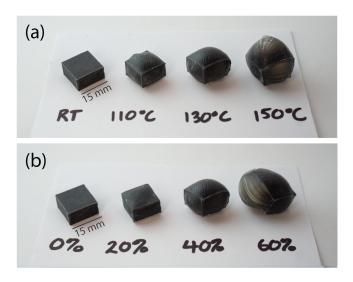
Figure 7: The degree of bulging may be modulated with (a) heating temperature (fixing microsphere slurry concentration at 40 wt% and heating time at 5 minutes) or (b) microsphere slurry concentration (fixing heating temperature at 130°C and heating time at 5 minutes).
