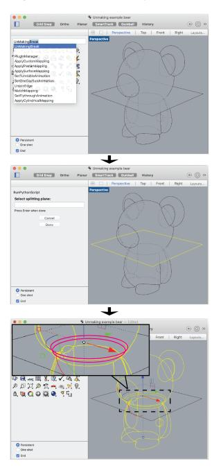
Figure 8: A custom *Rhino* macro allows the designer to define surfaces along which a 3D model should break and generates modified meshes that can be exported as *.stl* models to be sliced, 3D printed, and unmade. An inset highlights the added mesh boundaries in pink.
