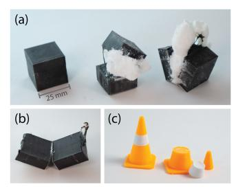
Figure 5: (a) PLA cubes can be split parallel to print layers OR perpendicular to print layers. (b) The surfaces of the split PLA pieces after microspheres are brushed off are smooth. (c) Splitting may be used to separate multi-color (or multimaterial) artifacts cleanly into their constituent parts for recycling.
