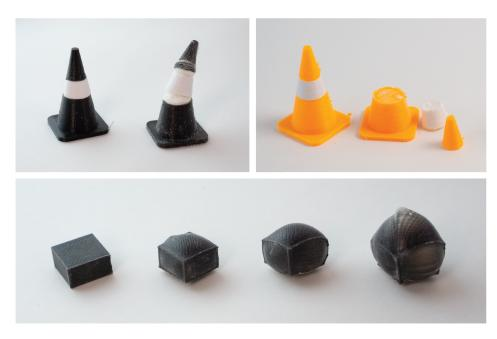
Figure 1: Exemplar unmaking designs achieved using multi-material 3D printing, exhibiting splitting (top left), breaking (top right), and bulging (bottom)
