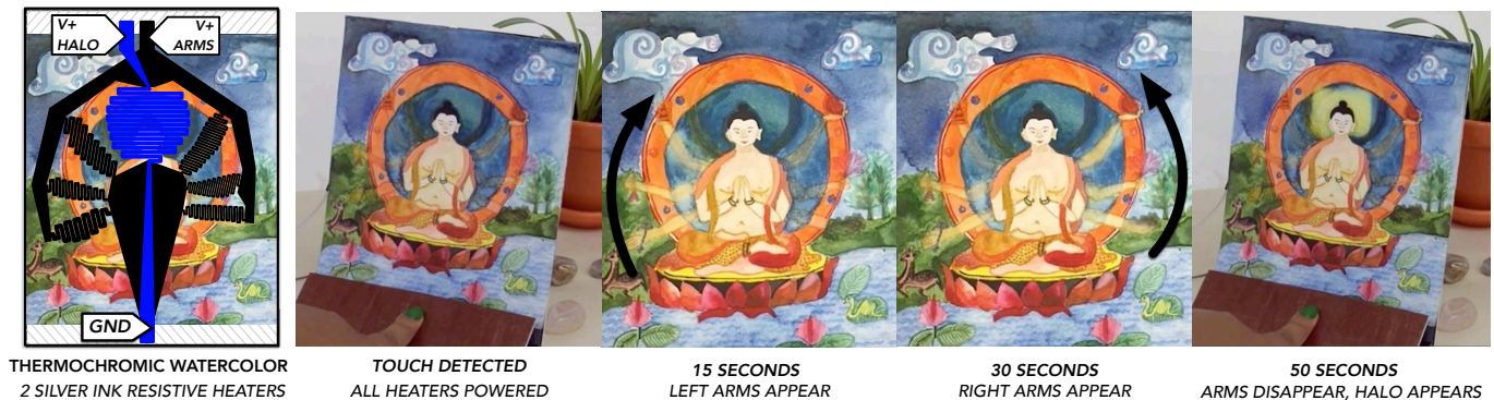
Figure 1. Two joule (resistive) heaters are designed relative to a thermochromic watercolor composition. By constructing resistors in parallel, heat is applied to select regions of the composition but generated at different rates triggering different thermochromic changes over time. The final artifact is a representation of a non-emissive display and "timer" for prayer and reflection.
