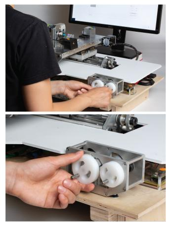
Figure 1. Top: the Turn-By-Wire system consists of a lathe, haptic feedback handwheels, and a graphical user interface. Bottom: detailed view of the handwheels used to directly and digitally control the lathe.
