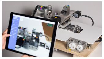
Figure 10. In our AR envisionment, a tablet computer renders a virtual wood material into the lathe (round, tan colored cylinder on screen). No material is physically loaded into the lathe.
