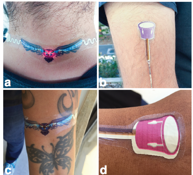
Figure 12. Representative Pictures of Skintillates Devices in User Study. Participants were free to apply the Skintillates tattoo on any body location. Example applied body locations include a) neck, and b) arm. c) Skintillates LED displays used in the study utilize small 0603 LED parts, which allows the Skintillates tattoo to retain its conformal profile. d) Skintillates resistive sensor used in the study worn on arm.
