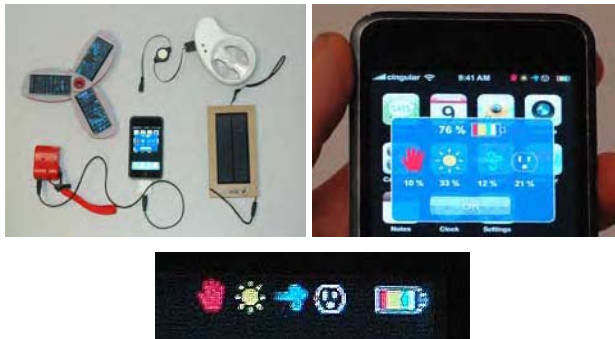
Figure 2. Interactive microgeneration devices and iPod battery icons ('hand', 'sun', 'wind' and 'outlet' power).
