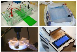
Figure 2. Gel electrophoresis box in a professional lab (top left) and assembled from scratch at London Hackspace (top right); Dremelfuge developed by Indie Biotech, image source www.indiebiotech.com (bottom left); OpenPCR kit for replicating DNA (bottom right).
