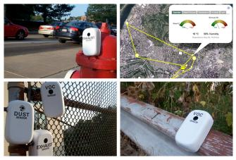
Figure 1. Exhaust sensor attached to fire hydrant near busy street (top left); map of exhaust data gathered by parents (top right); dust, exhaust and VOC sensors attached to bridge (bottom left); VOC sensor on park railing (bottom right).
