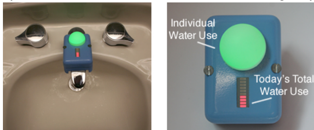
Figure 3. Faucet display mounted onto a public bathroom faucet (left) and each part of the display labeled (right).
