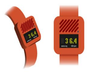
It is not uncommon for people to use Bluetooth headsets (exposed to ambient air) while their mobile phone is in their bag or pocket (not exposed to ambient air). Similarly, we can imagine the use of various Bluetooth based air quality sensors attached to clothing, body, or backpacks for sampling the ambient atmosphere. We are also in the process of developing a wristwatch version of the hardware with a numeric output on a watch face. A sketch of this design concept is shown (Figure 7).
